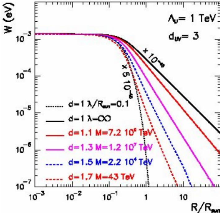
Function  $W(r)$  due to the density of protons (or electrons) in the Sun as a function of the distance from the solar center in units of the solar radius,  $R_{\odot}$ , for various values of the dimension  $d$  and the mass scale  $M$ . We take  $\Lambda_u = 1 \text{ TeV}$  and  $d_{UV} = 3$ . For comparison, we show the value of the  $W(r)$  function for a Coulomb-type ( $d = 1$ ) long-range force with range  $\lambda = 0.1 R_{\odot}$  and with the same strength at the center of the Sun.
