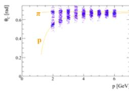
A preliminary study on the HMPID detector resolution of two close tracks addresses the capabilities of HMPID for HBT. Fast MC simulations of tracks in a close phase space (in different momentum bins) are performed, including complete simulation of HMPID response in a 0.2T magnetic field. The studied momentum regions are shown with the extracted  $\theta_c$  for particle identification.
