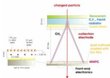
HMPID exploits the properties of Cherenkov light and large surface CsI photocathodes to identify charged particles on track by track basis. Charged particles crossing the detector produce Cherenkov photons in the radiator. These photons, detected by a pad-segmented cathode MWPC, produce a typical ring pattern. A dedicated algorithm of pattern recognition gives the information on the mean Cherenkov photon emission angle. Then PID could be performed.
