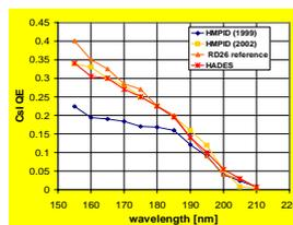
CsI quantum efficiency as a function of photon wavelength.
