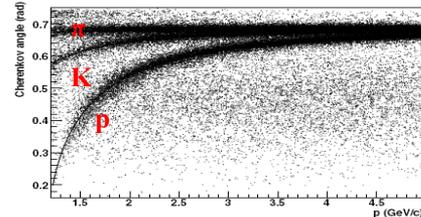
Particle identification in HMPID (upper panel) and the corresponding efficiency and contamination for pions, kaons and protons. (ALICE Physics Performance Report, Volume II)
