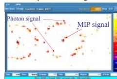
A display of rings from pions during test beam.
